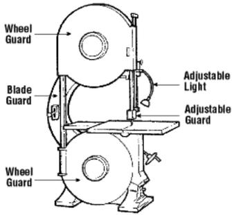
Band Saw - has a continuous blade and stroke, the blade travels around two pulleys. It is used to make curved or irregular cuts.
