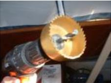
Hole saw– used with a drill for making large holes or cutting wheels.
