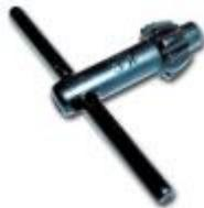
The chuck key is necessary to tighten drill bits in power drills. The gear on the chuck key meshes with the gear in the chuck of the drill to add torque when tightening.
