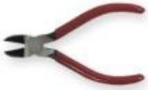
Diagonal cutting pliers— used to cut wire.
