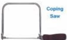
Coping Saw - it is used for cutting curves. The replaceable blade has fine teeth which point towards the handle.
