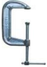
C-clamp– used to hold your material stationary on your work surface or while gluing.
