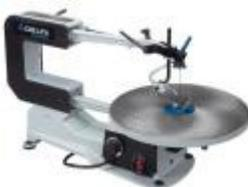
Scroll Saw / Jig Saw - cuts in reciprocating motion (up and down), cuts only on down stroke, used for cutting curves.
